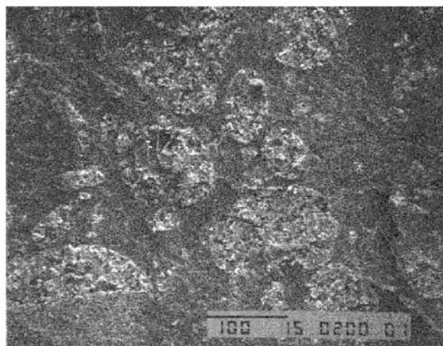
FIGURE 7 SEM micrograph of the fracture surface of R5.
